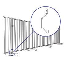
A further Heavy duty fencing couple should then be installed approximately 300mm down from the top of each panel joint, this should be left loose until the stabiliser is attached.
