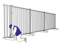
Remove the nut from the top Heavy Duty Hoarding Coupler and locate in place a Hoarding Stabiliser. Replace the nut on the hoarding coupler and tighten to fix stabiliser in position.
